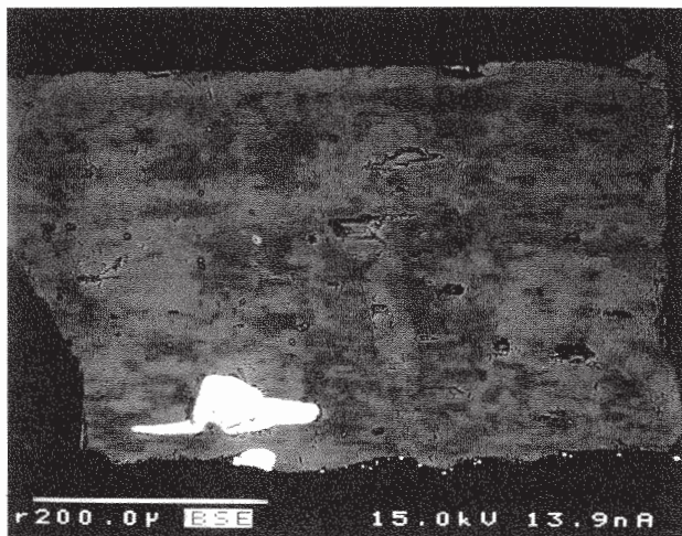
Photo 1. BSE image of tourmaline from metamorphosed fluorite layer. Euhedral crystal of tourmaline contains small fluorite inclusions (bright). Dravite-schorl domains (dark) within the Mg-rich schorl crystal
