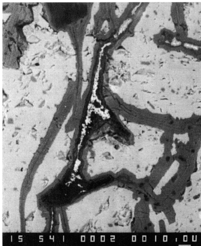
Fig. 1 Alteration products of the Peerless stannite (sample PPK-1). Grey veinlets – unknown Cu, Fe, Zn-phosphosilicate (or a multiphase mixture); black – carbonate of Cu; white in black – cassiterite.
