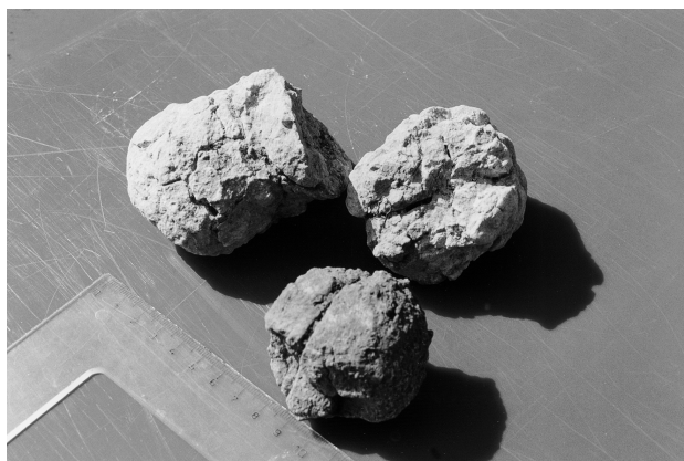
Fig. 7 Isolated caliche nodules. Note the cracks that are probably due to the displacive growth of carbonate minerals. Červený lom Quarry.
