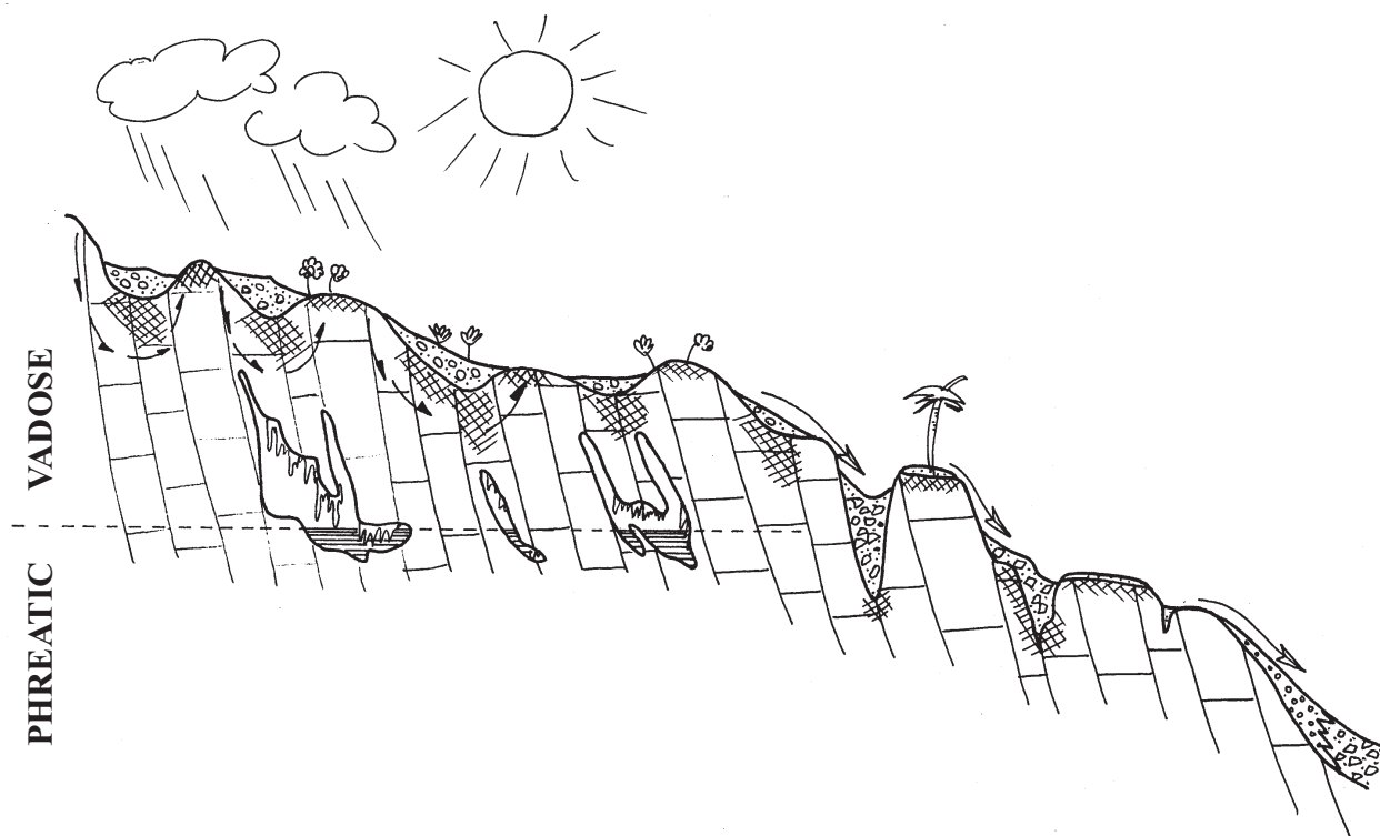
Fig. 15 Sketch showing conceptual model for the origin of the “white beds” of the Barrandian area. The full arrows show the movement of surface water in the upper vadose zone as predicted by “ per ascendum ” model of caliche formation. The vertical extent of the resulting alteration zone is shown as hatched areas. The open arrows point to the redeposition of the alteration crust into local depressions of the paleo-relief (paleokarst depressions?). The deeper vadose to phreatic caves and/or surface karst landforms often develop ponecontemporaneously with the caliche profiles, especially under less arid climatic conditions.
