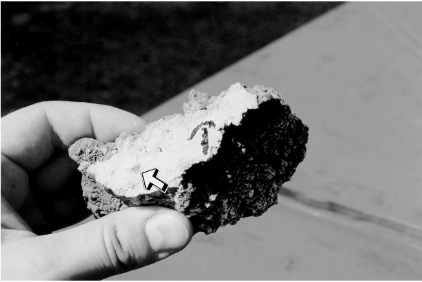
Fig. 8 Fragment of the platy caliche. Indistinct laminar structure and a small carbonate intraclast (open arrow) embedded within the bed can be recognized. Dark arrow points to the top of the bed. Červený lom Quarry.
