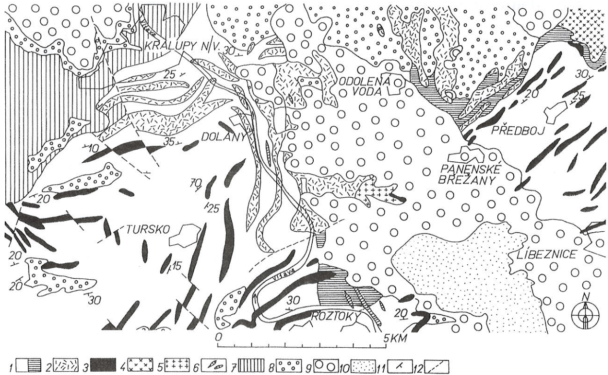
Fig. 1. Distribution of lensoid silicite bodies in the area north of Prague (after A. Matějka in Ciniburk 1962, (simplified) 1 – Proterozoic greywackes and shales; 2 – spilitic rocks; 3 – lydites; 4 – granodiorite, diorite; 5 – ditto; 6 – porphyrite, porphyre; 7 – Permocarboneous; 8 – Cenomanian; 9 – Turonian rocks; 10 – Quarternary; 11 – faults; 12 – foliation
