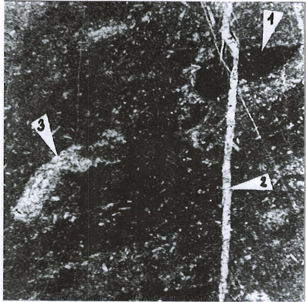
2. Type C: Microbioclastic calcisiltite with fine graded bedding, tiny calcite dykes and intraclasts of biomicrite. Zlíchov Formation (Zlíchovian), Hvíždalka quarry, grey colour 1 - intraclast, 2 - calcite dyke, 3 - piece of coral (Tabulata); Magnification: x8
