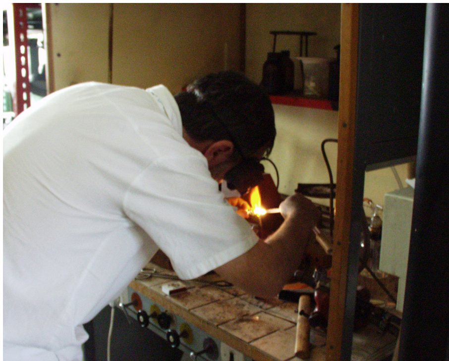
Fig. 2 Milan sealing silica glass tube in the Laboratory of Experimental Mineralogy of the Czech Geological Survey, Prague (March 2004). Photo by A. Vymazalová.
