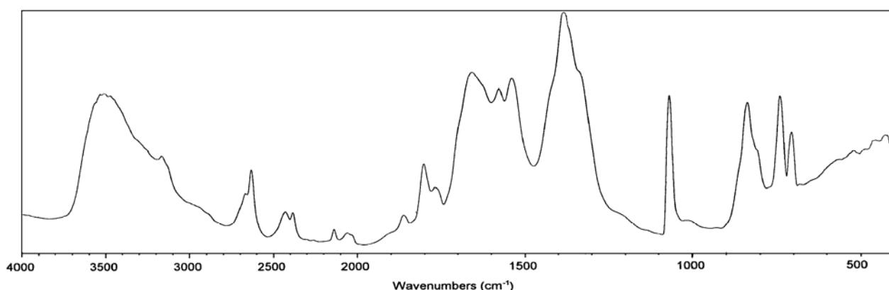
Infrared absorption spectrum (KBr tablet) of synthetic  $\text{Na}_4(\text{UO}_2)(\text{CO}_3)_3$
