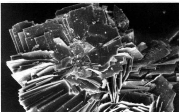
Aggregate of thin tabular crystals of the phase Ca-(VO)-AsO<sub>4</sub>. Magnification 90
