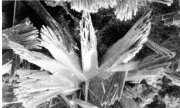
Aggregate of acicular crystals of the phase **MOASO**. Magnification 150
