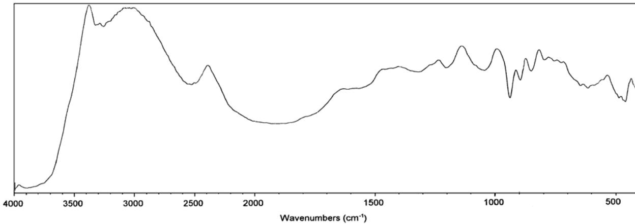
Infrared absorption spectrum (KBr tablet) of Ca(H<sub>2</sub>AsO<sub>4</sub>)<sub>2</sub> from Jáchymov.
