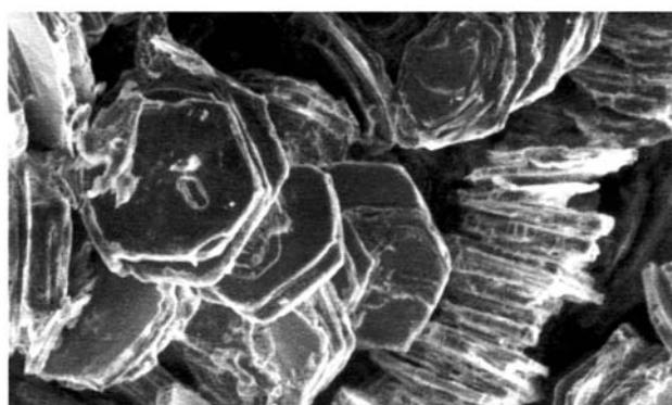
Hexagonal crystals of the phase Mg-AsO<sub>4</sub>-H<sub>2</sub>O. Magnification 150**The phase: Na<sub>4</sub>(UO<sub>2</sub>)(CO<sub>3</sub>)<sub>3</sub>**
