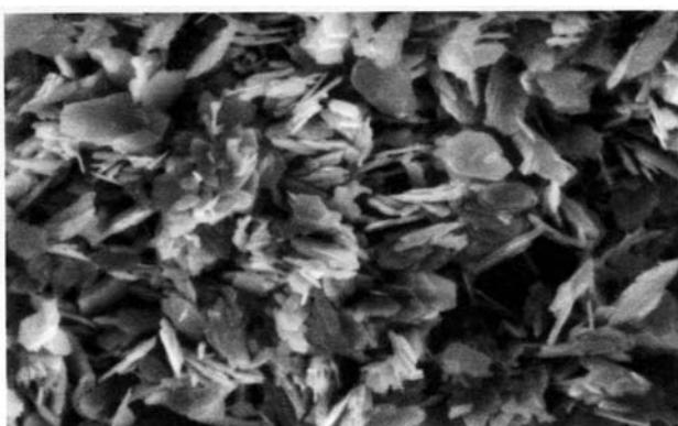
Aggregate of minute tabular crystals of the phase Fe-AsO<sub>4</sub>-H<sub>2</sub>O (2). Magnification 1000
