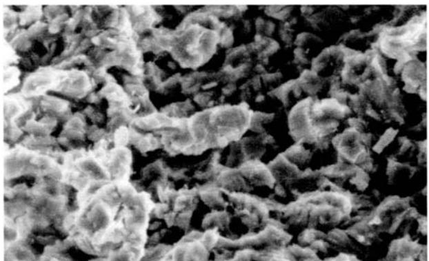
Detail of earthy, poorly defined crystals of the phase "pseudo-zippeite (Mg)". Magnification 800
