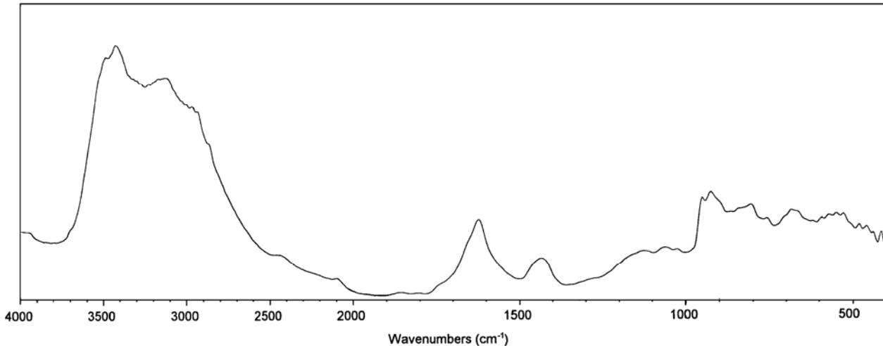
*Infrared absorption spectrum (KBr tablet) of MOASO from Jáchymov*
