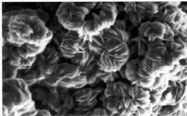
Rosette-shaped aggregates of tabular crystals of the phase **CAS**.
