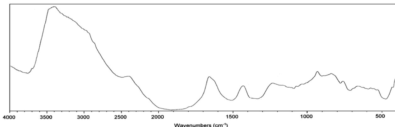
*Infrared absorption spectrum (KBr tablet) of  $\text{U}(\text{HAsO}_4)_2 \cdot 4 \text{ H}_2\text{O}$  from Jáchymov*
