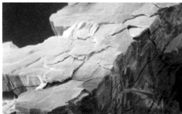
Fractured aggregate of the phase Cu-AsO<sub>4</sub>-H<sub>2</sub>O(2). Magnification 400
