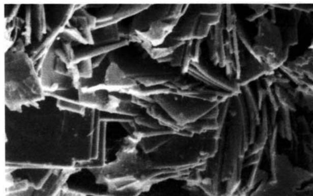
Aggregate of tetragonal tabular crystals of the phase Ni(UO<sub>2</sub>)<sub>2</sub>(AsO<sub>4</sub>)<sub>2</sub>·6-8H<sub>2</sub>O. Magnification 500**The phase: PbO-UO<sub>3</sub>-H<sub>2</sub>O**
