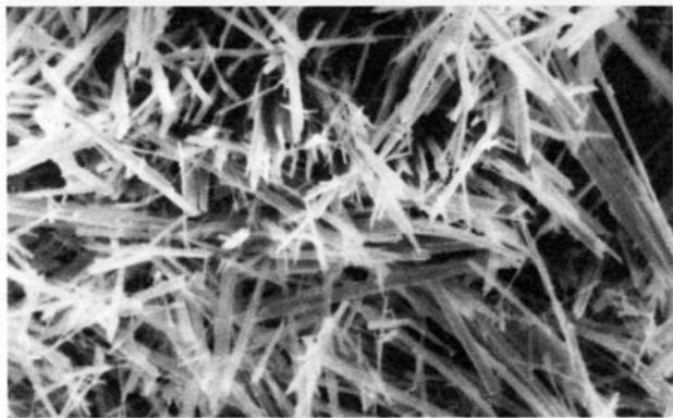
Acicular crystals of the phase Ca-Mg-AsO<sub>4</sub>-H<sub>2</sub>O. Magnification 500
