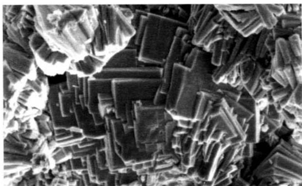
Aggregate of rectangular tabular crystals of the phase  $\text{U}(\text{HAsO}_4)_2 \cdot 4 \text{ H}_2\text{O}$ . Magnification 500
