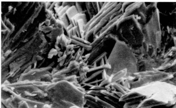
Aggregate of tabular crystals of "Mg-villyaellenite". Magnification 500
