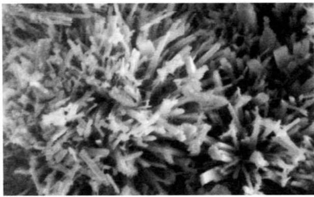
Aggregate of minute acicular crystals of the phase Fe-AsO<sub>4</sub>-H<sub>2</sub>O (1). Magnification 900
