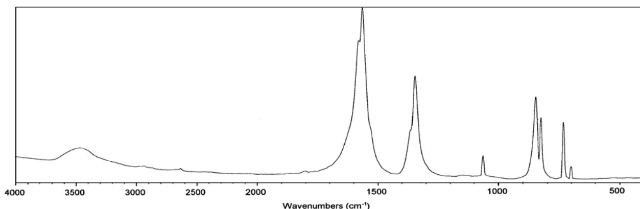
Infrared absorption spectrum (drift) of synthetic  $\text{Na}_4(\text{UO}_2)(\text{CO}_3)_3$ .
