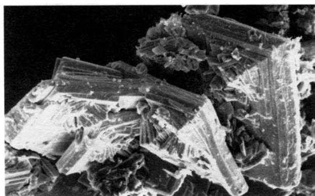
Tabular crystals of the phase  $\text{U}(\text{HAsO}_4)_2 \cdot 4 \text{ H}_2\text{O}$ . Magnification 250
