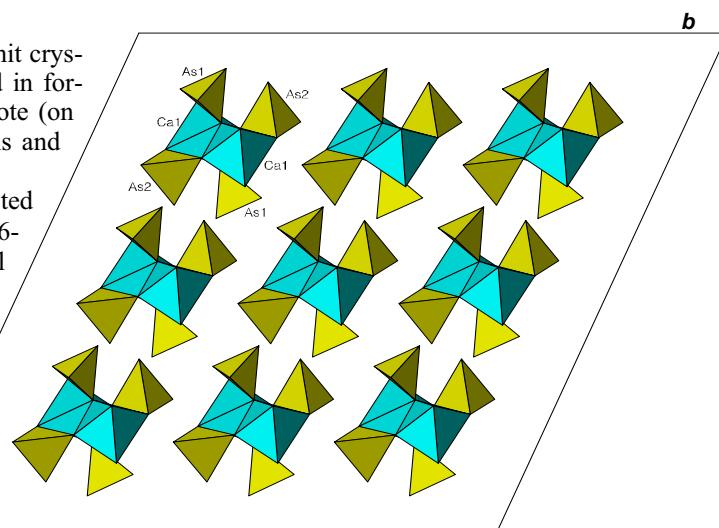
Projection of the  $\text{Ca}(\text{H}_2\text{AsO}_4)_2$  crystal structure onto  $ab$  plane.
