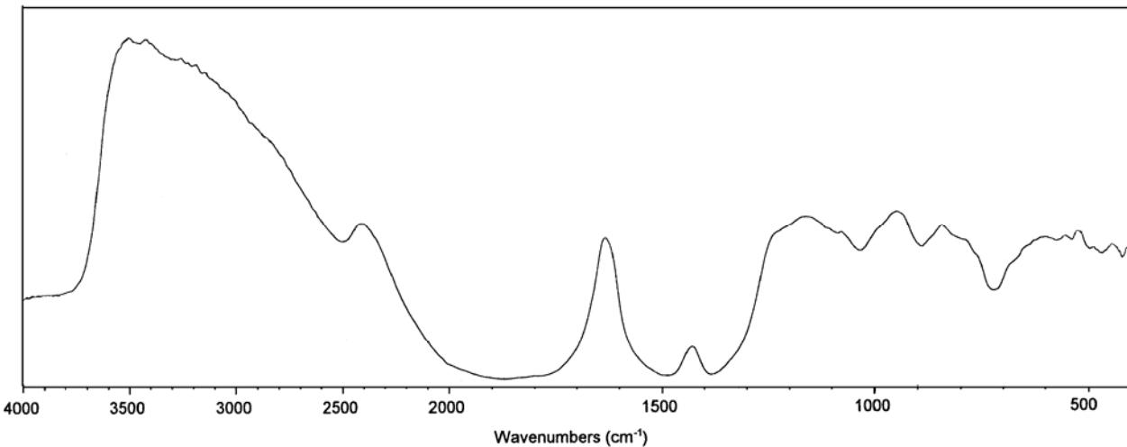
Infrared absorption spectrum (KBr tablet) of "Fe-AsO<sub>4</sub>-H<sub>2</sub>O(2)" from Jáchymov.
