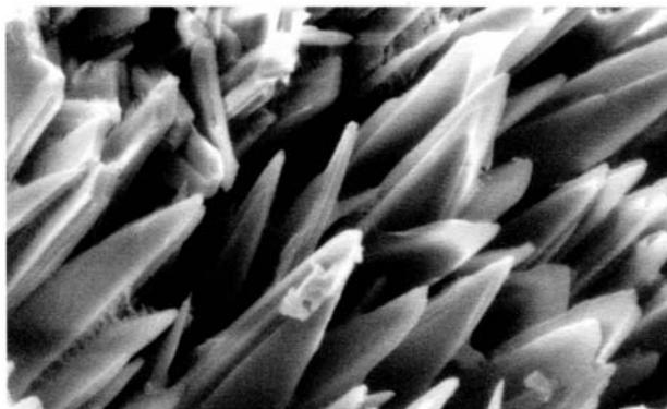
Radiating aggregates of crystals of the phase Cu-AsO<sub>4</sub>-H<sub>2</sub>O(3). Magnification 1000
