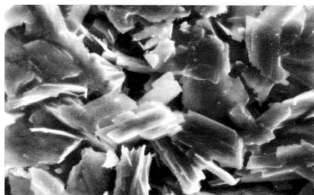
Imperfectly developed orthorhombic crystals of the phase Cu-AsO<sub>4</sub>-H<sub>2</sub>O (1). Magnification 1000
