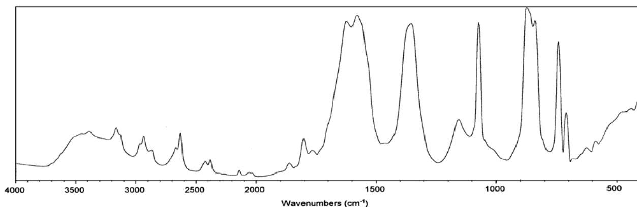
Infrared absorption spectrum (KBr tablet) of  $\text{Na}_4(\text{UO}_2)(\text{CO}_3)_3$  from Jáchymov.
