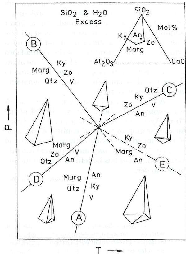
Fig. 3. Univariant curves pertinent to the stability of margarite plus quartz in the system  $\text{H}_2\text{O}-\text{CaO}-\text{Al}_2\text{O}_3-\text{SiO}_2$  according to Storre - Nitsch (1974) and Jenkins (1984). Invariant point involves the phases anorthite (An), kyanite (Ky), margarite (Marg), zoisite (Zo) and  $\text{H}_2\text{O}$  (V). Dash-dot boundary is metastable in quartz (Qtz) excess system
